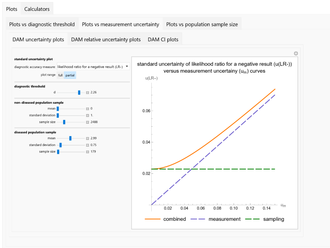
Figure 6. Plots vs. measurement uncertainty module, DAM uncertainty submodule screenshot. Standard combined, sampling, and measurement uncertainty of likelihood ratio for a negative test result ( u(LR^-) ) versus standard measurement uncertainty ( u_m ) curve plot, with the settings shown at the left.
