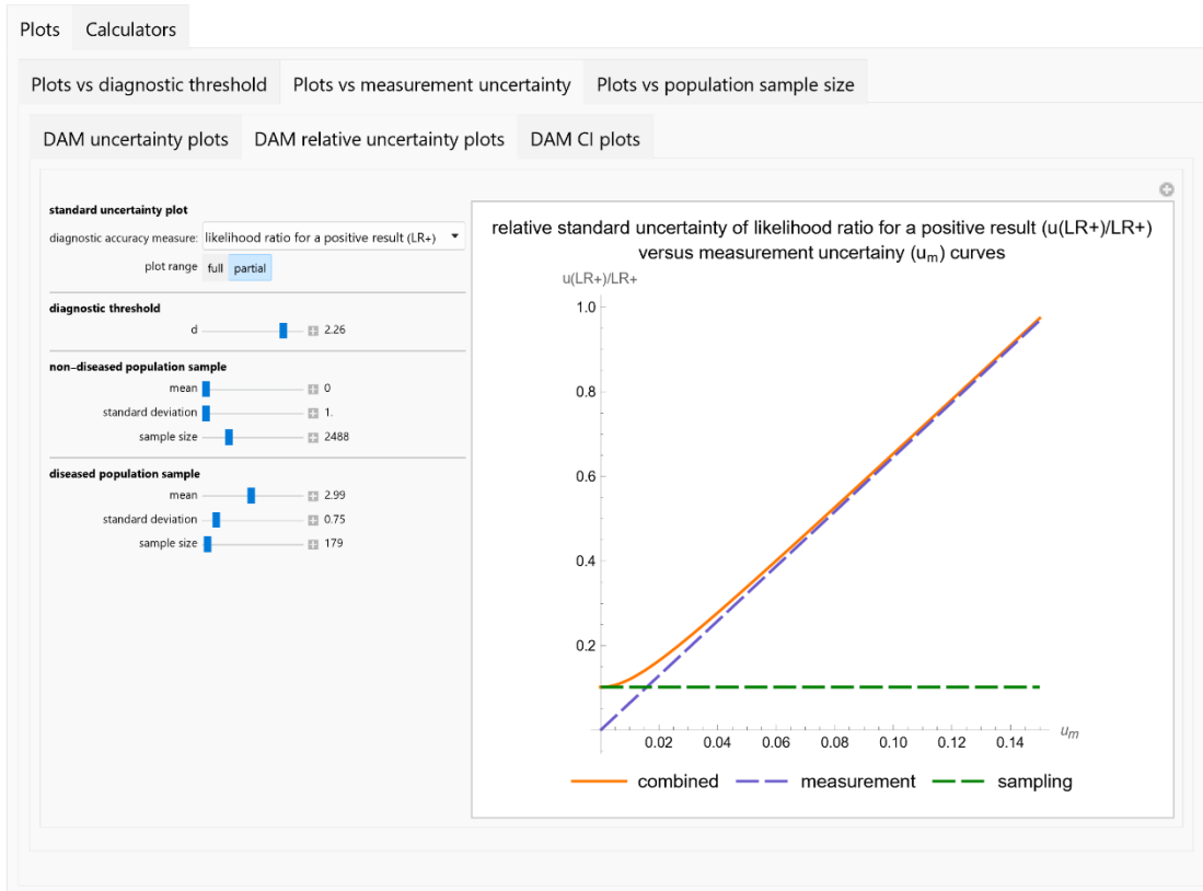
Figure 7. Plots vs. measurement uncertainty module, DAM relative uncertainty submodule screenshot. The relative standard combined, sampling, and measurement uncertainty of likelihood ratio for a positive test result ( u(LR+) ) vs. measurement uncertainty ( u_m ) curves plot, with the settings shown at the left.
